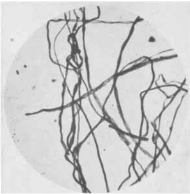
Fig. 2. Allylcellulose in Xylol-Medium, \text{H}_2\text{SO}_4 50° Bé.
